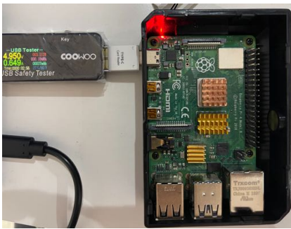
Fig. 9. Deployment on Raspberry Pi with power meter.
